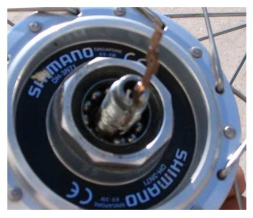
Break the lock nut from the cone on the non drive side of the hub and remove both. Then using a  $32 \, \text{mm}$  wrench grab the large nut on the drive side of the hub pictured below and turn counterclockwise. This will take a little force, brace the wheel against your body for a good grip.
