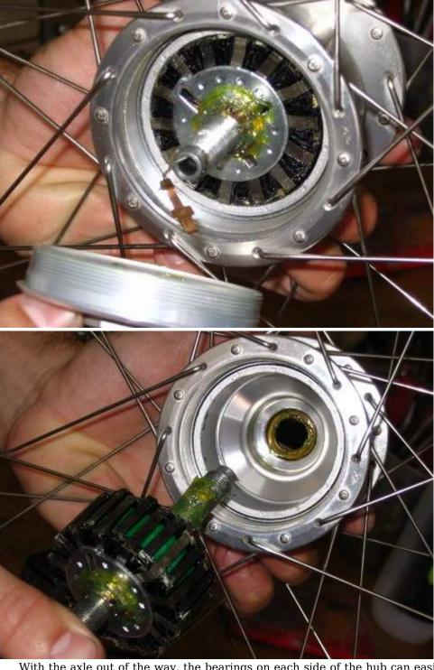
With the axle out of the way, the bearings on each side of the hub can easily be removed and the cups cleaned and inspected. Remove all the old grease and repack, replacing bearings as necessary.
