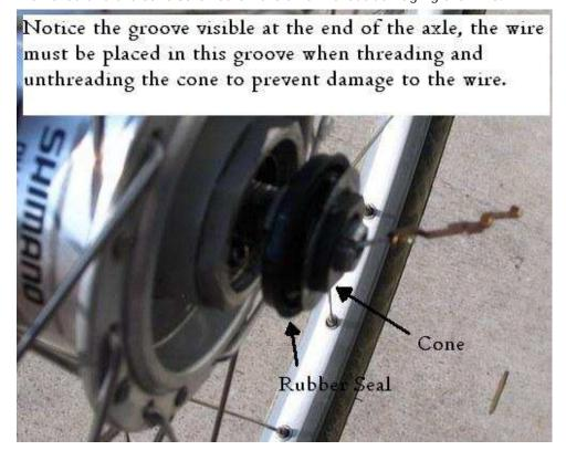
At this point the ball bearings on the drive side are exposed, but they're not easily accessible and you'll find it hard to clean the cups of the hub well unless we remove the axle.
