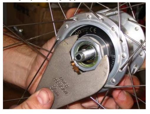
Now the inner assembly of the dynamo can can be removed.
