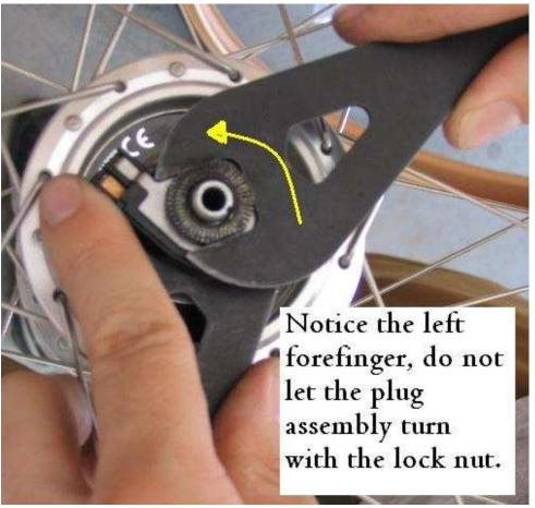
Now that the lock nut is removed, you can begin to take apart the plug assembly and remove the current wire from the plug. Below is a picture of the parts on the drive side of the hub. Parts 3 though 8 constitute the plug assembly along with the current wire and the connector that is soldered to the current wire.
